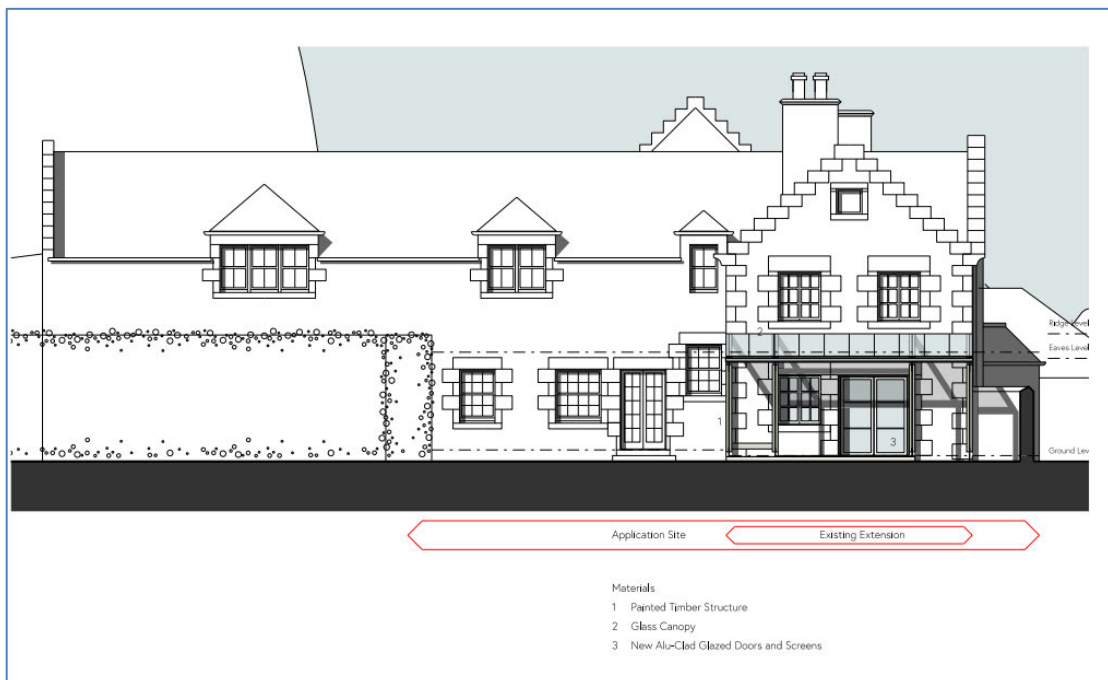
Figure 6: Proposed alterations to the rear (north) modern elevation of the appellant's property
